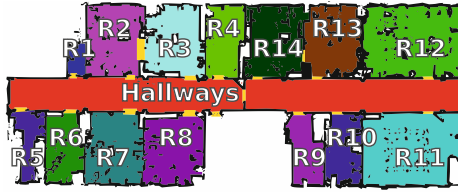
Fig. 3. Data set used for evaluation. The occupancy grid map of a building at the University of Freiburg. Sixteen different classes are labeled: 14 rooms, hallway and passages.
