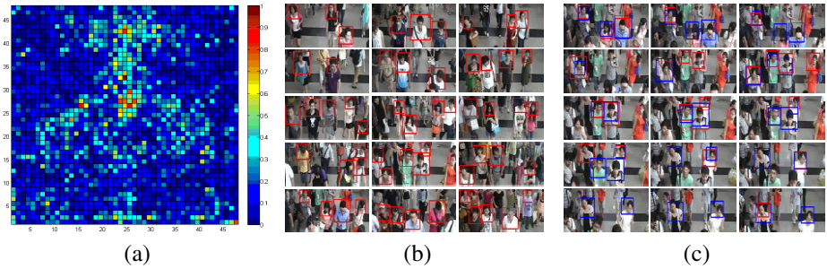
Fig. 6. (a) Visualize spatial support of the trained detector, (b) Examples of detection results for different levels of person density. The size of the bounding boxes shows the size of detected pedestrians, (c) An example tracking sequences. The blue boxes are the tracking results; the red boxes are the detecting results in current frame.
