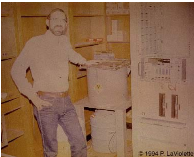
Figure 5. The author standing next to the Portland State University gamma ray detector used in his neutron activation analysis study of ice age polar dust.
