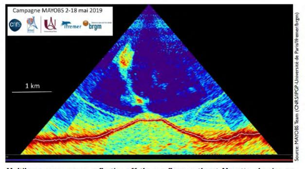
Multibeam sonar waves, reflecting off the sea floor southeast Mayotte, showing an 800-m-tall volcane (red profile), with a 5 km diameter and a rising gas-rich plume
