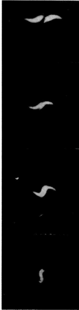
Figure 2.13. The evolution of two plasmoids fired at each other across a magnetic field (courtesy W. Bostick).
