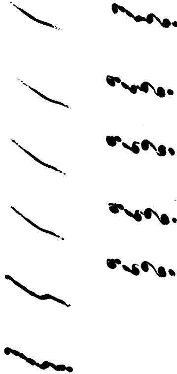
Figure 2.15. Laboratory simulated aurora. Voltage (current) increases continuously from top to bottom in each column.
