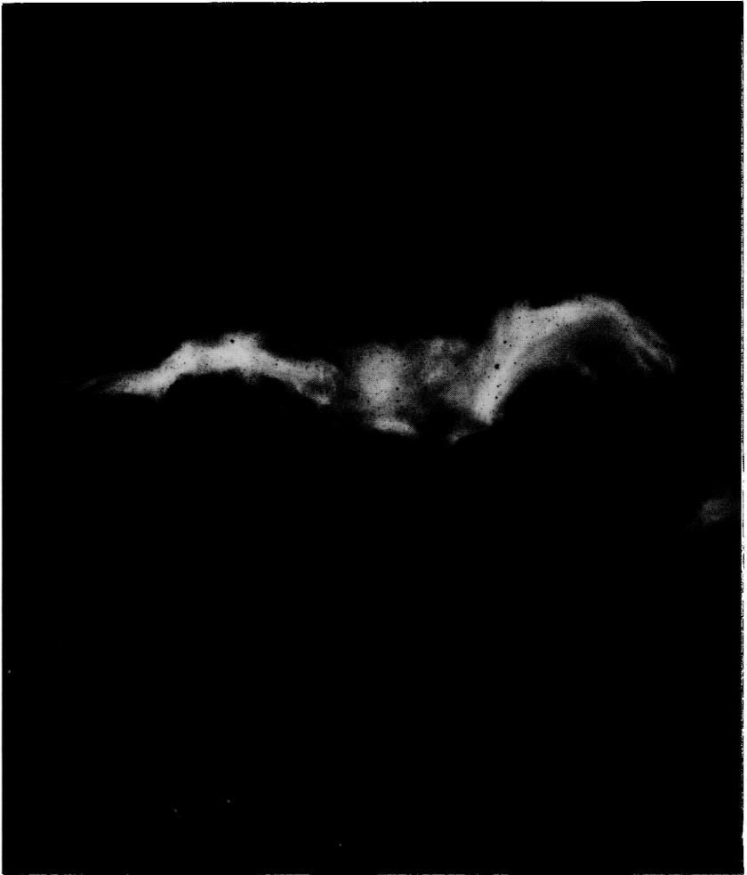
Figure 1.2. Filamentary plasma structure produced by “exploding” titanium wires within a 10 terawatt pulsed-power generator. The photograph was taken with a pin-hole X ray camera.
