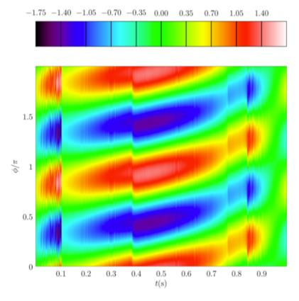
Simulated integrated Mirnov signal detected by a toroidal array of pickup when an n=2 I-coil current of 4.2 kA is applied to our model DIII-D plasma equilibrium. The relative phase between the currents flowing in the upper and the lower sections of the I-coil is ramped linearly on a time-scale of 1 s.
