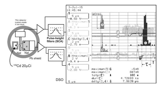
**Figure 6.** Gamma-ray experiment in tandem geometry using <sup>109</sup>Cd. Counters and computer interfaces are not shown. DSO screen is annotated.
