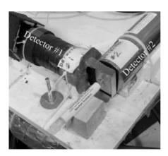
**Figure 5.** Two sodium iodide gamma-ray detectors in tandem geometry. Detector #1 is a custom-made 4 mm thick slab.
