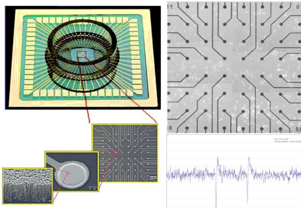
Fig. 2. A microelectrode array (MEA) commercially available from Multichannel Systems (upper left). 60 electrodes are arranged in an 8 x 8 grid spaced 200 um apart (lower left). The upper right panel shows neurons cultured on an array and lower left, and example of two spontaneous action potentials recorded
