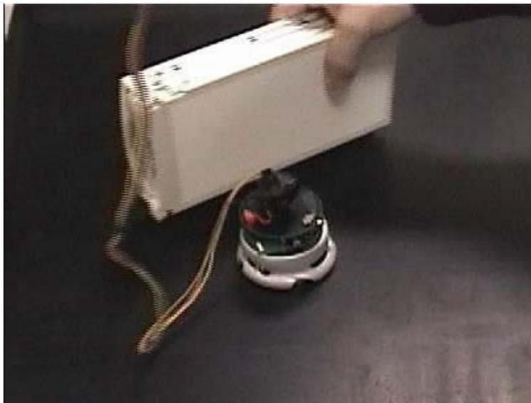
Fig. 7 Collision avoidance of Khepera II robot with living neuronal network (E18D96).
