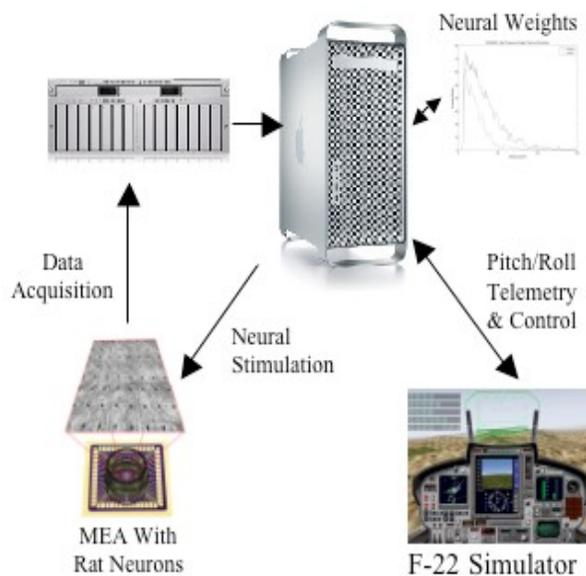
Fig. 1. Schematic of Neural Flight Control System using living rat cortical neurons for pitch and roll control.
