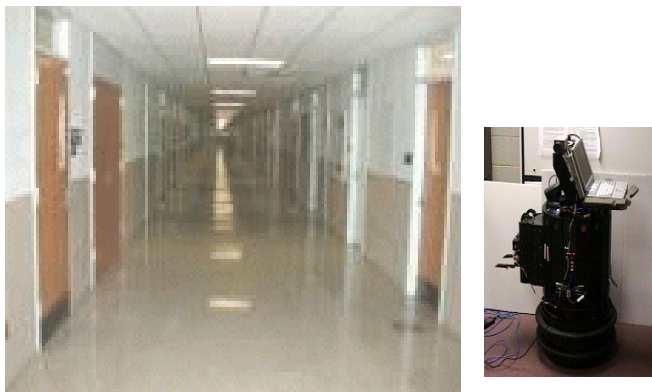
Fig. 2. The corridor on the left is a section of the MSU engineering building. Pavlov, the robot on the right, uses 16 sonar sensors to navigate the whole engineering building.
