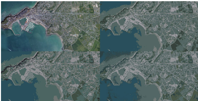
Fig. 3. From left to right, and from top to bottom : The original image 1131 \times 575 pixels, the result of our algorithm, the result using energy equation (8) and \beta = 1 , the result using energy equation (9) and \beta = 1
