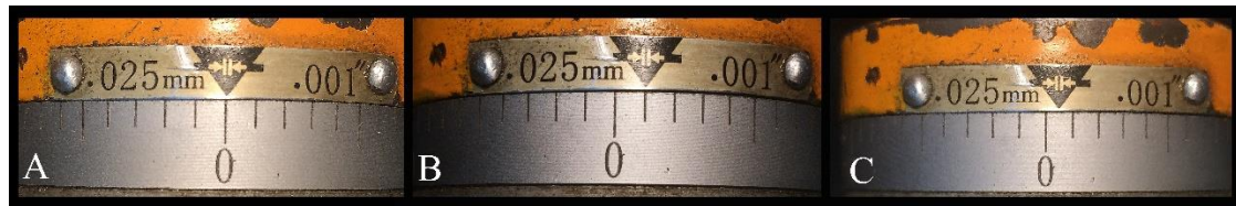
Figure 6: Close up of the micrometer dial of the tool post slide hand-wheel of a conventional lathe. Each line of the micrometer dial changes the tool post slide position by 0.025mm. Note that in any position between two lines, the movement of the tool post slide could not be defined.
