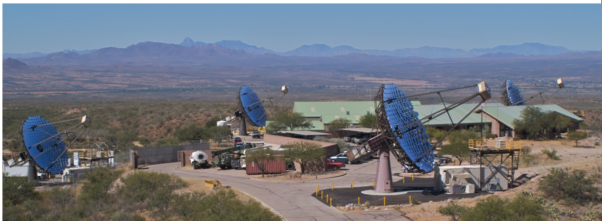
FIGURE 8.9 The VERITAS atmospheric Cherenkov telescope array for gamma-ray astronomy on Mount Hopkins in southern Arizona. SOURCE: Steve Criswell, Smithsonian Astrophysical Observatory.
