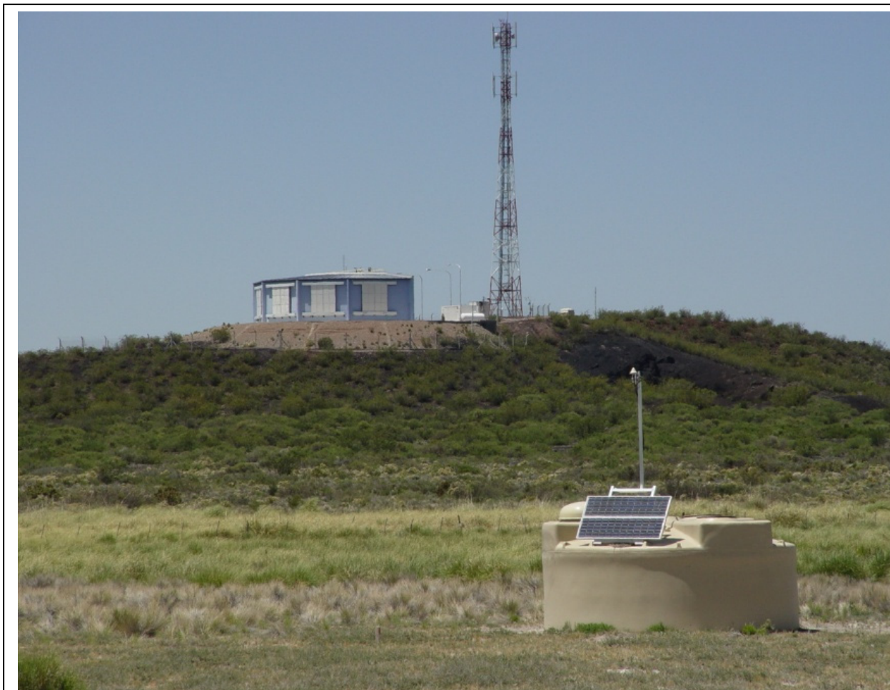
FIGURE 8.10 Pierre Auger Observatory of Ultra-High Energy Cosmic Rays in Mendoza Province, Argentina. Shown is one of the particle detector tanks of the 1660 units covering 3,000 square kilometers and one of the four fluorescence telescopes which overlook the array. SOURCE: Courtesy of the Pierre Auger Observatory.
