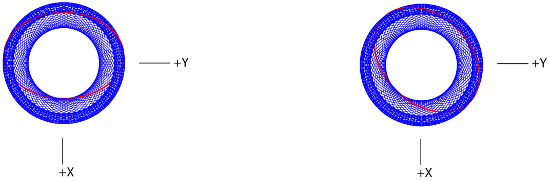
Figure 1.14. The current pattern given by Eq. (1.104) shown with 6 degree increments of \theta from the perspective of looking along the z -axis. The great circle current loop that served as a basis element that was initially in the xy -plane is shown as red.
