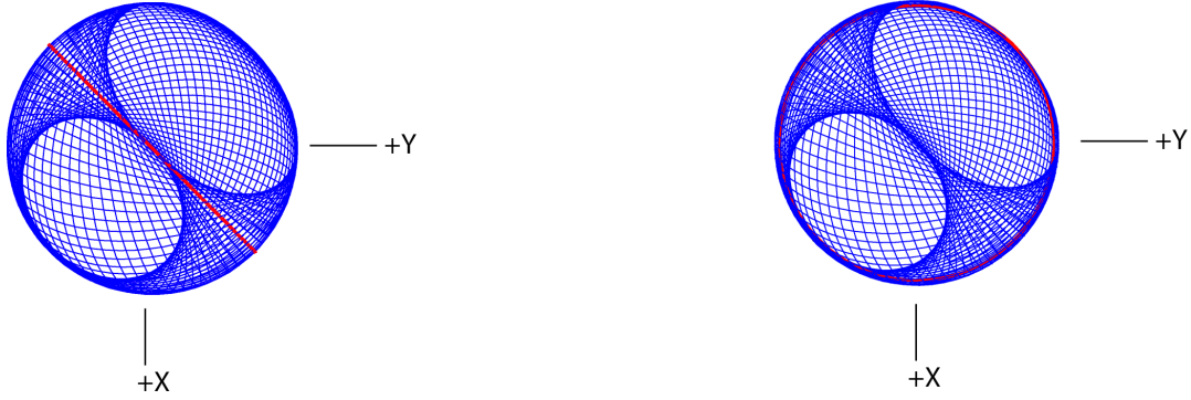
Figure 1.11. A representation of the z-axis perspective view of the OCVF shown in Figure 1.10 with 30 vectors overlaid giving the direction of the current of each great circle element.
